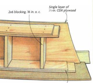
Bottom plate (two layers of 1/2-in. CDX plywood)
