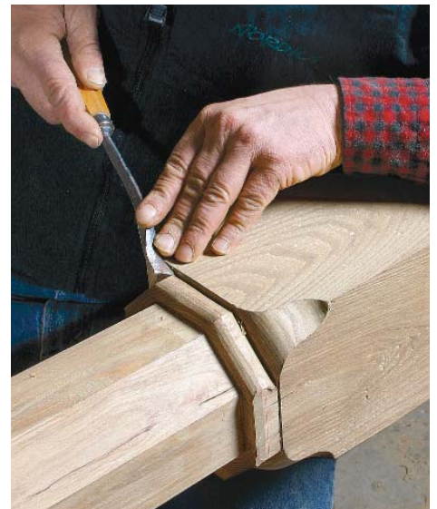
Razor-sharp tools for hand-carved details. To create the carved details at the top and bottom of the octagon, flat chisels pare down the convex surfaces (photo center), and a curve-bladed gouge shapes the concave surfaces (photo right).
